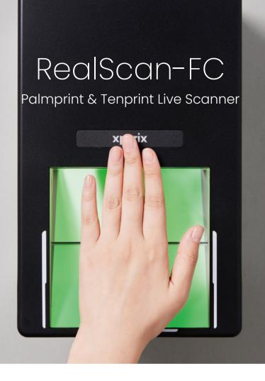
RealScan-FC is an all-in-one palmprint live scanner for capturing various types of fingerprints and palmprints, including slaps, flats, rolls, palms, and writer's palms. Featuring Xperix's cutting-edge optical & biometric technologies, it is capable of capturing the highest quality images regardless of the physical condition of hands.
