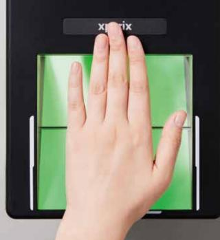
RealScan-FC is an all-in-one palmprint live scanner for capturing various types of fingerprints and palmprints, including slaps, flats, rolls, palms, and writer's palms. Featuring Xperix's cutting-edge optical & biometric technologies, it is capable of capturing the highest quality images regardless of the physical condition of hands.
